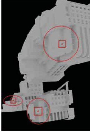
Figure 4: Render showing areas of reduced accuracy and modeler level of detail due to restrictions with the aerial LIDAR data coverage.
